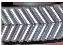
High precision herringbone gear
